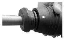
Slide the front of the chuck toward the body of the tool to insert, lock, and release an SDS Max bit
