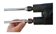
This mixer comes with two mixing paddles. Each is marked on the shaft for either the left or right mixer collar. The mixer collars are also plainly marked left or right. Simply insert the correct paddle into the collar and screw the collar down until tight.
