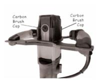
This product has two externally accessible brush assemblies that should be checked periodically for wear. Using a flat head screwdriver, remove the brush cap. The brush assembly is spring-loaded and will pop out when removing the brush cap. Remove the brush assembly (brush and spring). Check for wear on the carbon tips. Replace both brushes when either one has less than 1/4 inch length
