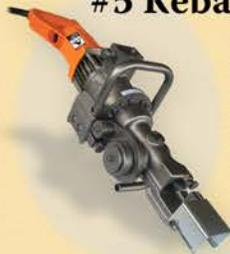
This combination tool provides jobsite cutting and bending all in one tool. The unique design provides the operator the ability to work rebar for in-place or stationary fabrication applications. The DBC-16H can easily bend #5 grade 60 rebar 180°.
