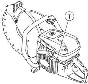
Rec. idle speed: 2700 rpm
