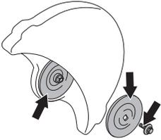
Do not use warped, notched, indented or dirty flange washers. Do not use different dimensions of flange washers.
