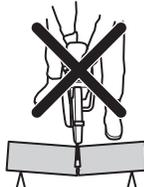
If the blade is pinched or stalled in the kickback zone, the reactive force will push the power cutter up and back towards the user in a rotating motion causing serious or even fatal injury. Be alert for potential movement of the work piece. If the work piece is not properly supported and shifts as you cut, it might pinch the blade and cause a kick back.
