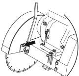
WARNING! Check that the blade, blade flange and blade shaft are undamaged. Clean the contact surfaces of the blade and the blade flange. Make sure the blade and the flanges are clean and free of dirt and debris before mounting the blade on the machine.
